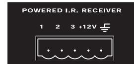
**Custom Installers:** The processor’s IR inputs sense modulated 38 kHz carrier, not demodulated data. With some control systems, an emitter face-to-face with an IR receiver may be needed.
